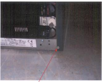
8) Remove Base Screw & lift off Side Panel. Note: Panel lifts upwards for approx 25mm before becoming free of guides.
