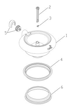
The major advantage of WaterGuard VI is that the air filter has now been relocated outside of the main body of the device – any water spills during bottle changing will not enter the filter media.
