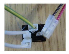
Connection of Wires to Relay
